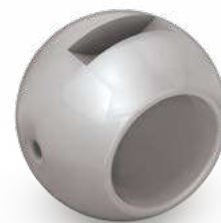
3 mm relief hole face the upstream
